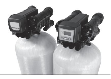
New top mounted valving and new GE controls make deionized water production easy and cost effective. These two column (one cation and one anion in series) systems are now available in five introductory flow rates and capacities, and include a monitoring system and sequential regeneration.
